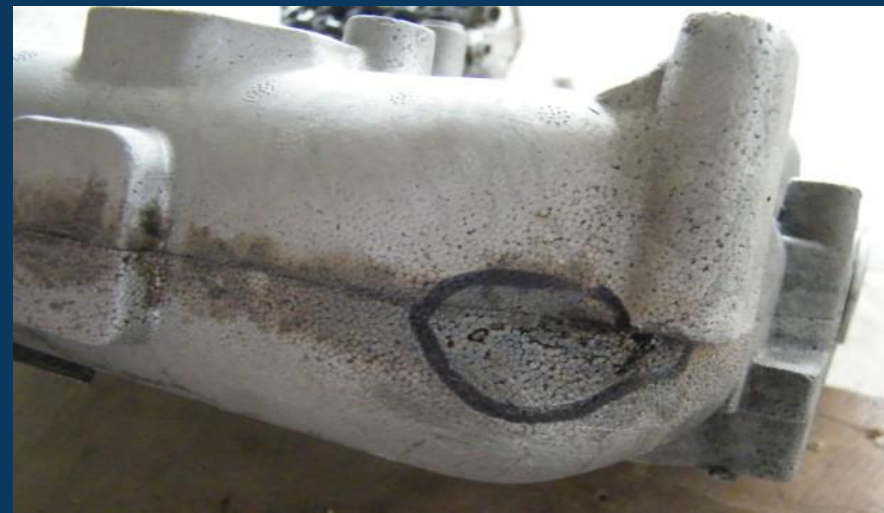
b. Castings produced from inferior foam patterns
